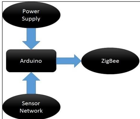
Fig. 1 Block diagram of sensing unit
