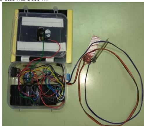
Fig. 3 Actual picture of sensing unit
