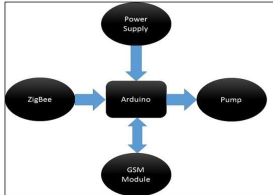
Fig. 4 Block diagram of control unit
