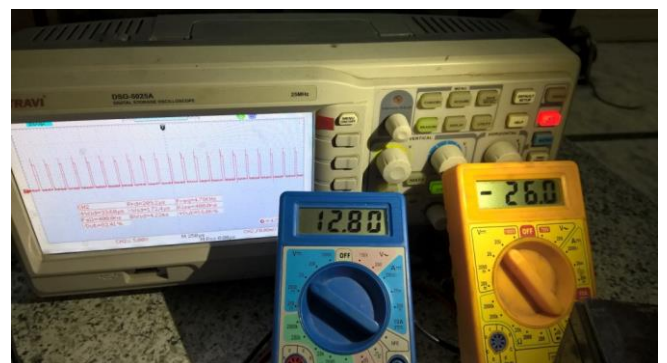
Fig 11. Input and output voltage at 25% duty cycle
