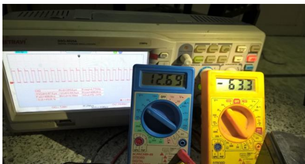
Fig 12. Input and output voltage at 60% duty cycle
