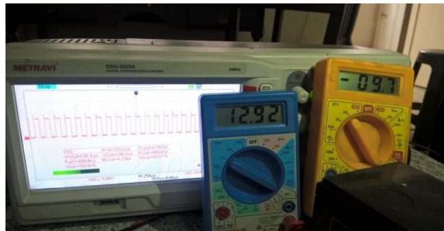
Fig 8. Input and output Voltage at 40% duty cycle
