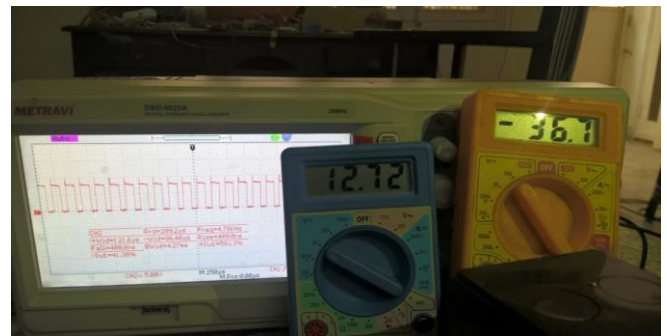
Fig 7. Input and output voltage at 58% duty cycle
