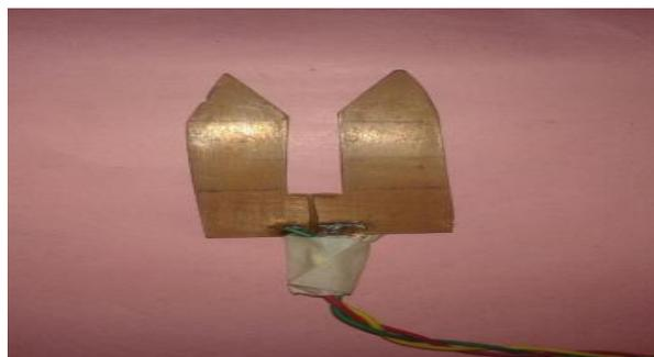
**Figure 4. Conductivity sensor.**
