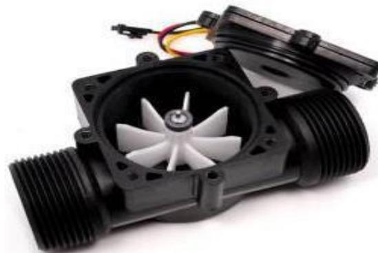
**Figure 6. Water flow sensor.**
