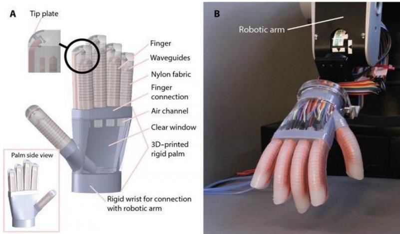
Optoelectronically innervated prosthetic hand was used to conduct various active sensation experiments inspired by the capabilities of a real hand. Our final demonstration used the prosthesis to feel the shape and softness of three tomatoes and select the ripe one
