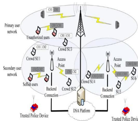
**Fig: 1.1 Dynamic Spectrum sensing**
