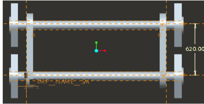
Fig. 5.3.2: Distance between two shafts for modified setup.
