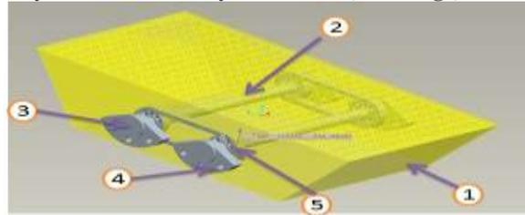
Fig. 5.3.3: Model of shakeout body, frame, bearings, Counterweights and shafts assembly.
