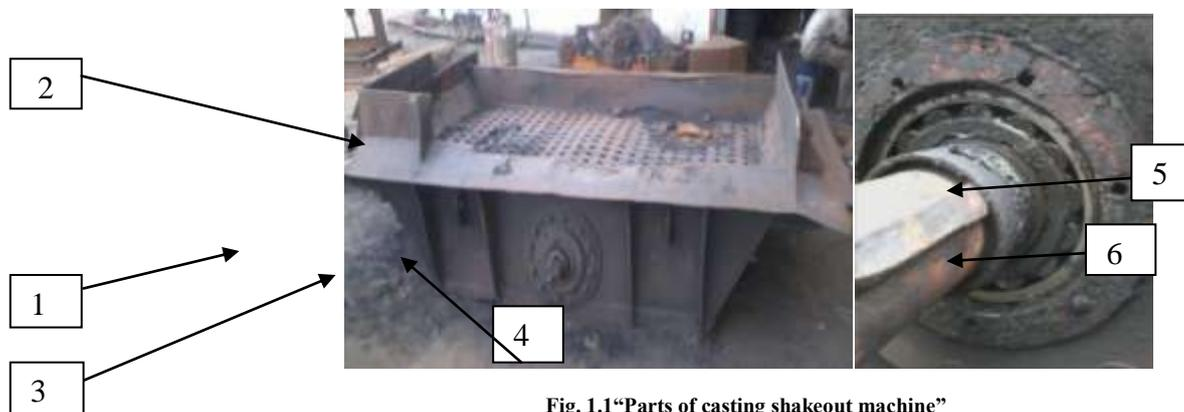
Fig. 1.1“Parts of casting shakeout machine”
