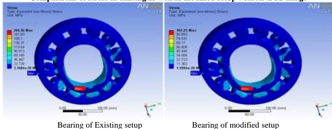
**Fig.6.2: Stress values in existing and modified setup**
