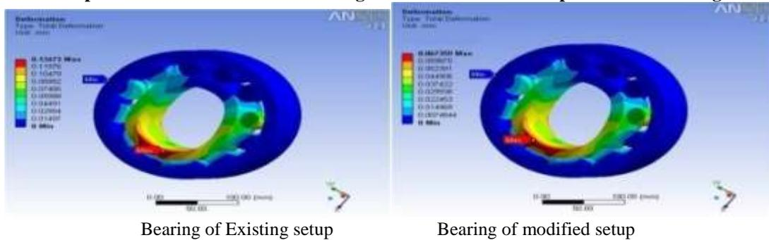
**Fig. 6.1: Deformation values in existing and modified setup**
