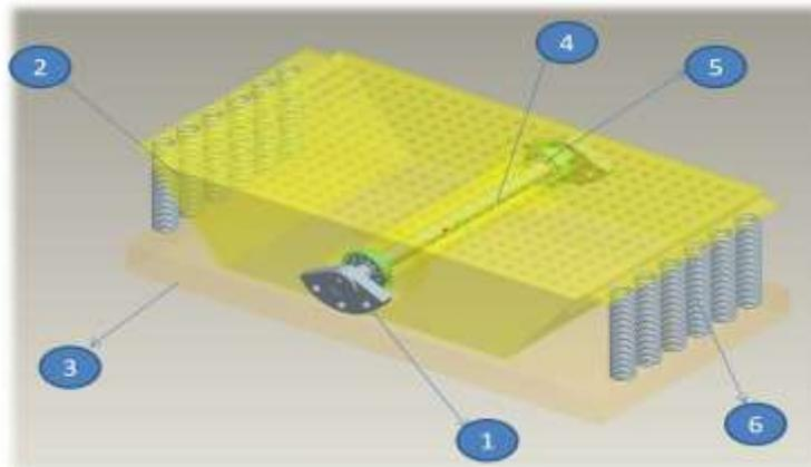
Fig. 5.1: Construction of Casting Shakeout
