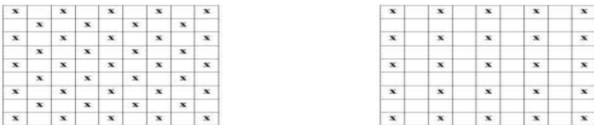
Fig4. The pixels which are marked by a cross are used to build the histogram. Left: One half of the pixels are used and Right: One 4 th of the pixels are used.
