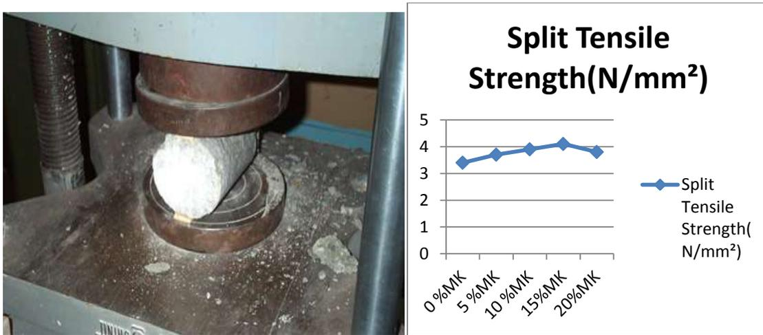
Fig. 3 Split Tensile testing
