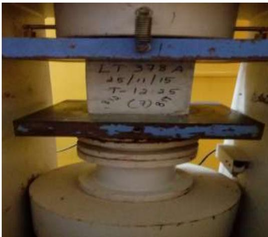
Fig.3 Compression testing
