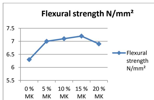
Fig.5 Flexural Strength testing
