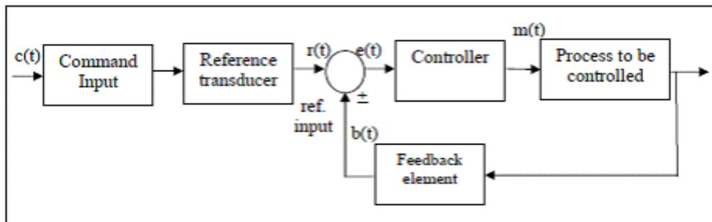
Figure 2 Block diagram of closed loop system
