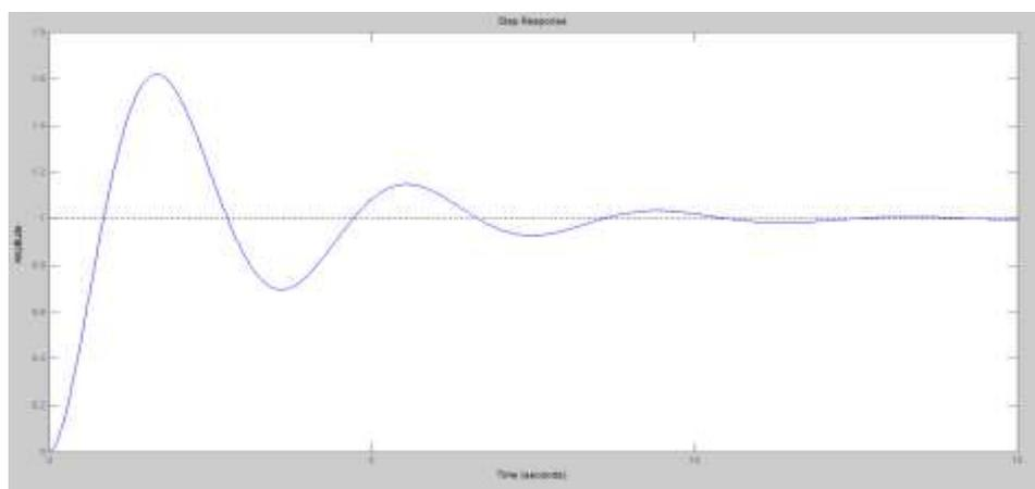
Figure 5.1 Unit step response of the system using Ziegler-Nichols method
