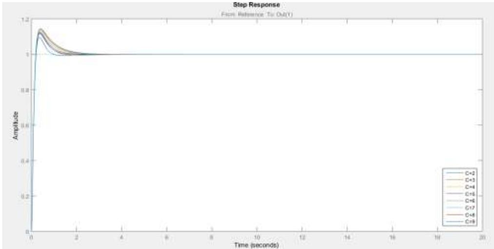
Figure 5.3 Output response of Concentration control of CSTR using PSO-Dependent PID controller
