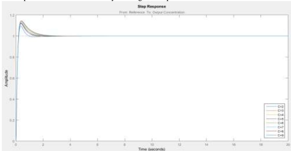
Figure 5.6 Output response of Concentration control of CSTR using HU-Dependent PID controller.
