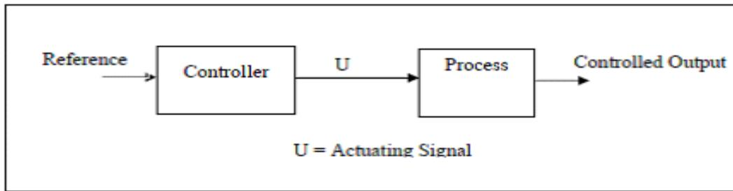
Figure 1 Block Diagram of Open Control System
