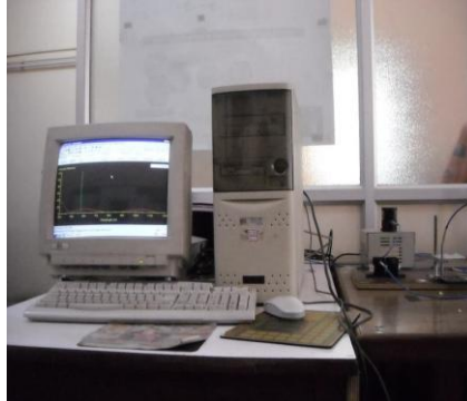
Fig.4.1 Experimental Arrangement of HR 4000CG High Resolution Spectrophotometer
