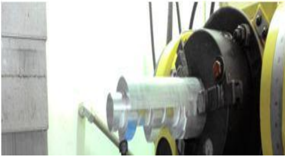
Fig. 22 After machining rest mill rotating the job to 180°
