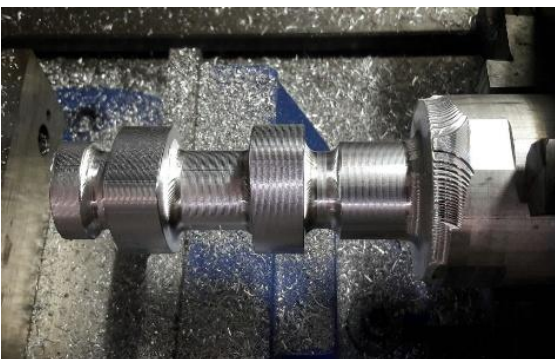
Fig. 25 Semi finishing completed
