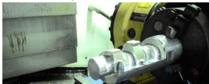
Fig. 21 After machining pocket on top segment
