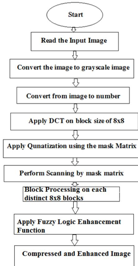
Figure 2: Implementation Block Diagram
