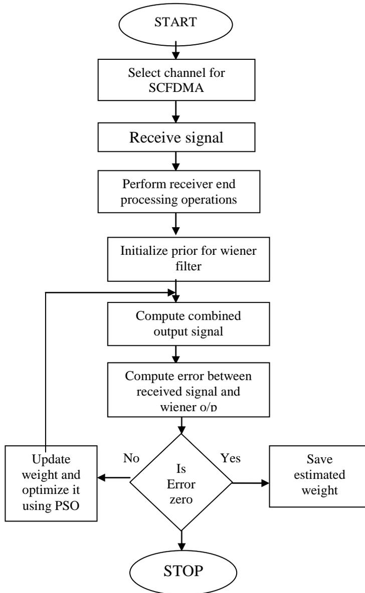
Fig.2 Flow chart of Adaptive channel estimation
