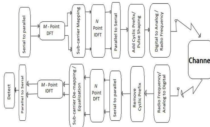
Fig. 1 Block diagram SCFDMA system
