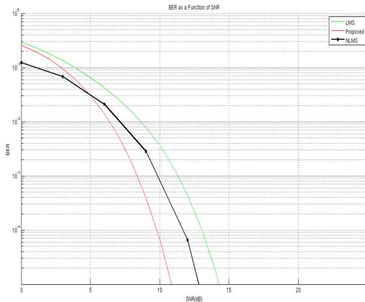
Fig 3: Comparison of different Estimation techniques in AWGN channel
