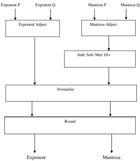
Fig1: Conceptual Overview of Floating Point Unit.
