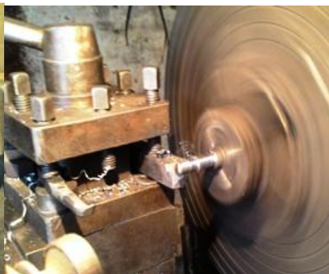
Fig. 2.2 Turning operation on specimens
