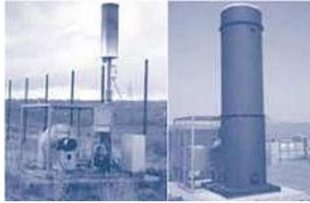
Figure 5: Open (left) and enclosed (right) flare.
