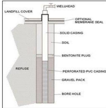
Figure 2: Gas extraction well
