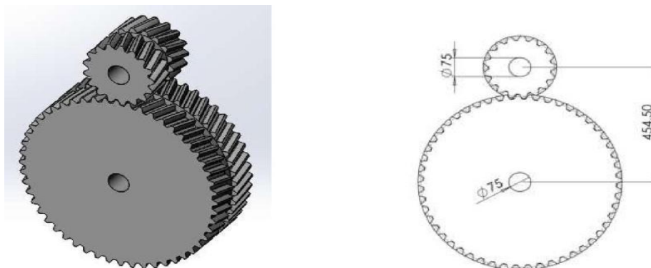
Fig. 3.3: Model & 2D Drawing of Gear Assembly of Module 12 Gear Dia 234 & Dia 675
