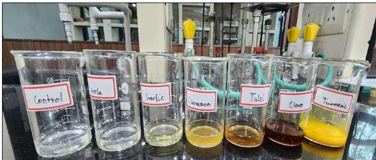
Figure 9: 10 cm 3 of Spice Extracts with 1 cm 3 of 0.1% (w/v) DCPIP aqueous solution
