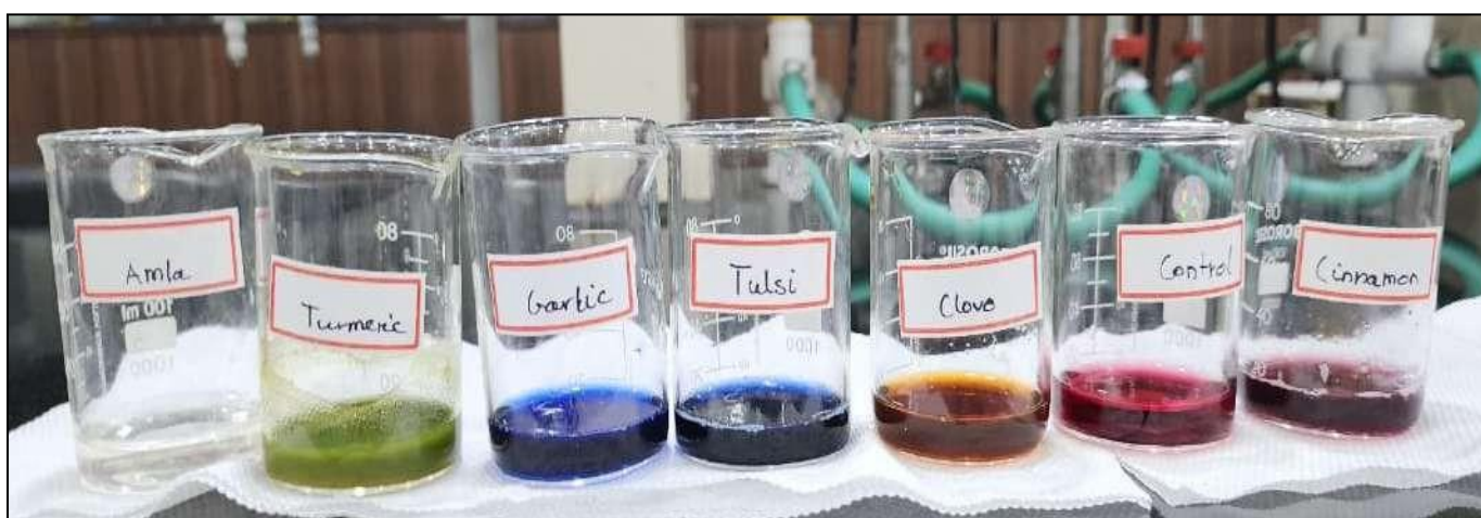
Figure 10: 10 cm 3 of Spice Extracts with 2 cm 3 of 0.1% (w/v) DCPIP aqueous solution
