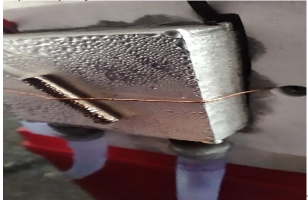
Fig.1. Extracted Water from Peltier Module
