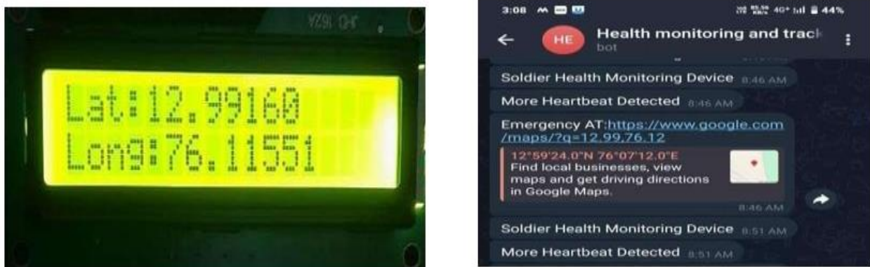
FIGURE-5: Detection and Display of Longitude and Latitude, Data (longitude and latitude) sent to the Telegram App
