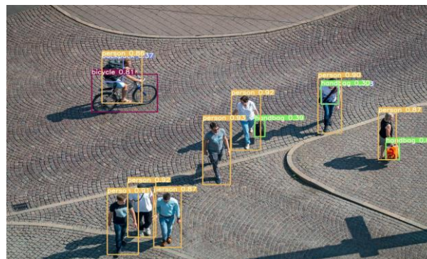
Fig.3. Object detection in real-time using YOLOv8
