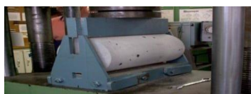
Fig 4: A Concrete cylinder undergoing Split Tensile Test
