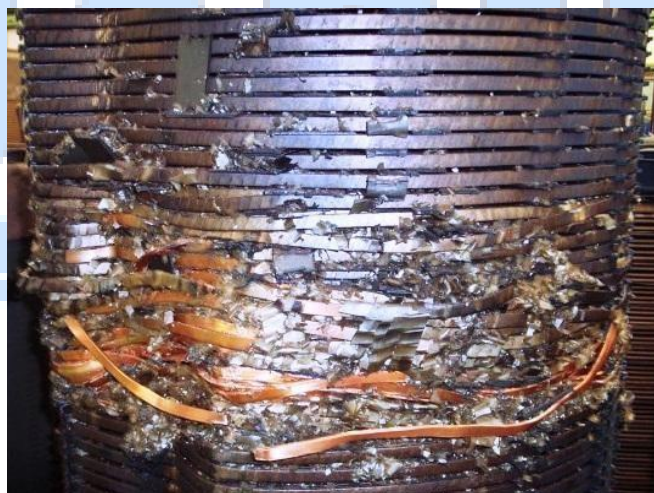
Fig.1: Example of catastrophic insulation failure of power transformer
