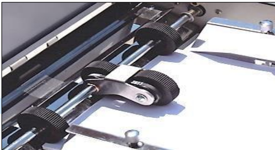
Fig.1 Paper Feeding and Paper Collecting Mechanism
