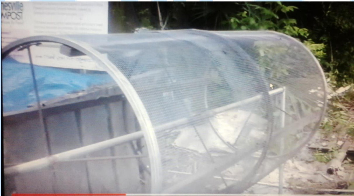
Fig 2 experimental setup of sand separator
