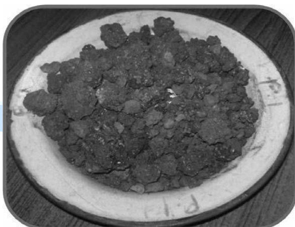
Pictorial View of Steel Slag Sample (Ref. from M/s.Jindal Steel Industries MIDC Sinnar,)
