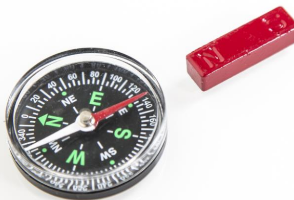
Fig. 3 Error in Magnetic compass due to proximity of a magnet
