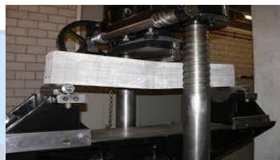
Fig 3: A Concrete beam undergoing flexural bending
