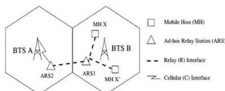
Fig. 3. A relaying example where MH X communicates with BTS through two ARSs [5]
