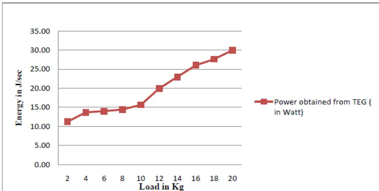
**Figure: 1.7** Graphical representations variation of power obtained from TEG with load variation of 2 kg to 20 kg at constant speed of 1300 RPM
