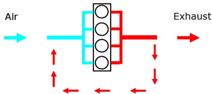
**Figure 1.2 Exhaust gas recirculation system**
