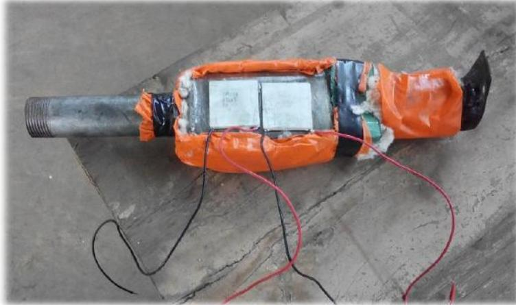
**Figure 1.4 Duct specification with TEG module**
