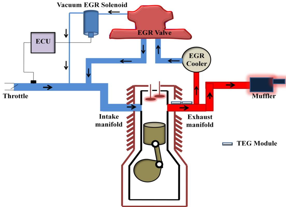
Figure 1.5 TEG and EGR system coupled with Engine
