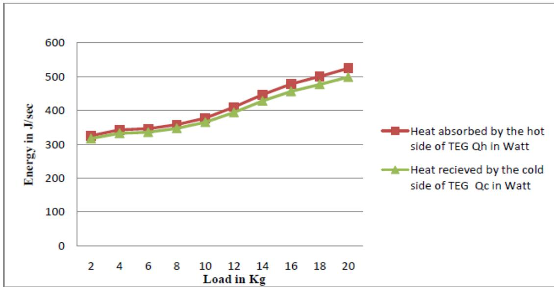
**Figure 1.6** Graphical representations of variation of heat absorbed by hot side of TEG and heat received by cold side of TEG with load variation of 2 kg to 20 kg at constant speed of 1300 RPM,
