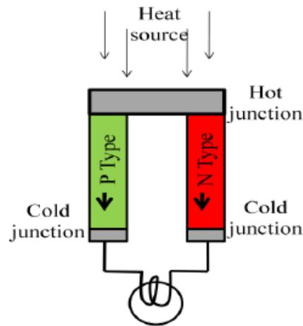
**Figure 1.3 Thermoelectric power generation**
