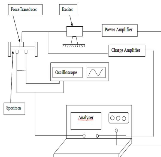
Figure 4 : Schematic Diagram of Experimental Setup
