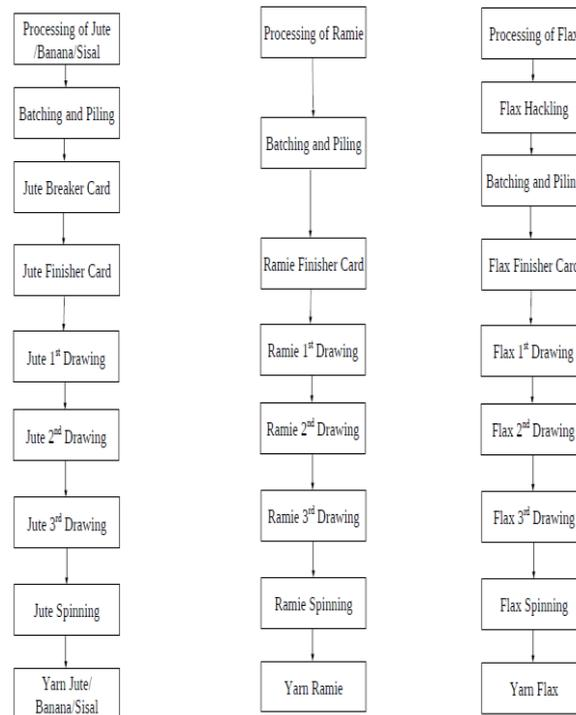
Fig.2. Processing Steps of Natural Fiber
