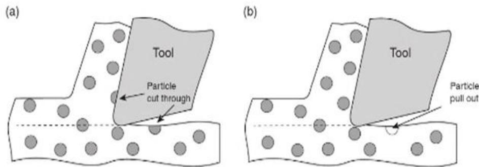
Figure 2.1 Schematic diagrams for cutting MMC's (a) particle cut through (b) particle pull out[12]
