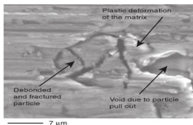
Figure 1: Scanning electron microscopy (SEM) image showing different deformation mechanism in a MMC[12]
