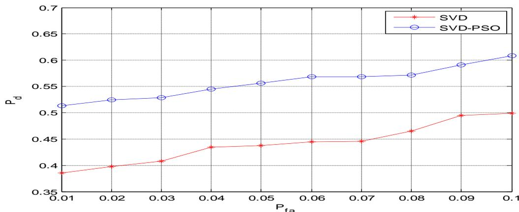
Figure 4. Comparative graph for probability of detection vs. probability of false alarm for SVD and SVD-PSO based detection algorithms
